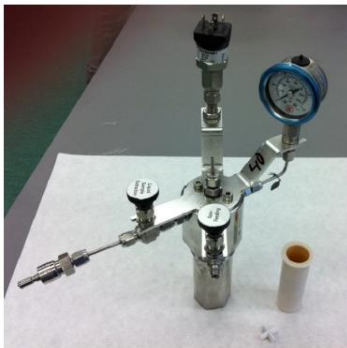
Figure S90. Standard autoclave used for the copolymerization reaction between CO 2 and epoxide(s).
