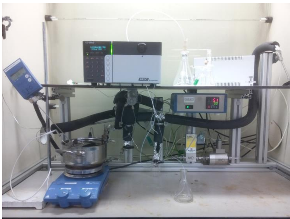
Figure S2. Picture of the capillary microreactor setup for the aerobic cross-dehydrogenative coupling of o -xylene.
