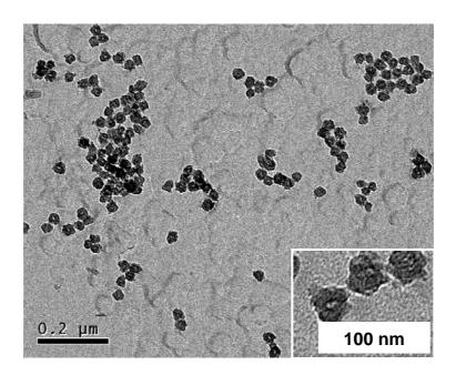
**Figure S2.** Transmission electron micrograph of hybrid copolymer-silica particles (the same particles as shown in Figure 2B, formed by 50 % quaternized PDPA $_{23}$ -PDMA $_{68}$  micelles) after redispersion in acidic solution at pH 2 with the aid of an ultrasonic bath.
