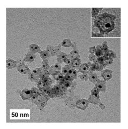
**Figure S5.** Transmission electron micrograph of hydrid copolymer-silica particles obtained by protonating the PDPA chains within the cores of the silica-coated micelles using HAuCl<sub>4</sub>, followed by in situ reduction using NaBH<sub>4</sub>. This experiment confirms that the PDPA chains remain located within the micelle cores after silica deposition, as expected.
