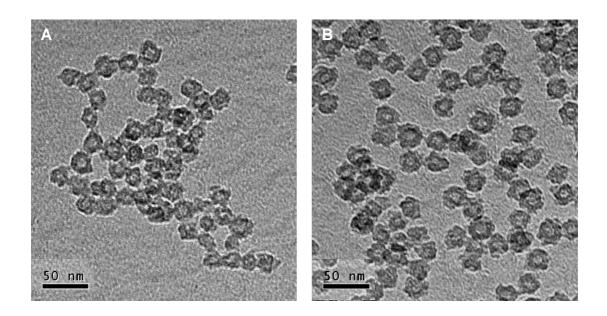
**Figure S3.** TEM images obtained for hybrid copolymer-silica particles using SCL micelles (50 % mean target degree of crosslinking by BIEE) as templates and a reduced excess of TMOS: (A) prepared by stirring a mixture of 2.0 mL of a 0.25 wt. % copolymer micelle solution with 58 mg TMOS for 20 min; (B) prepared by stirring a mixture of 2.0 mL of a 0.25 wt. % copolymer micelle solution with 116 mg TMOS for 20 min.
