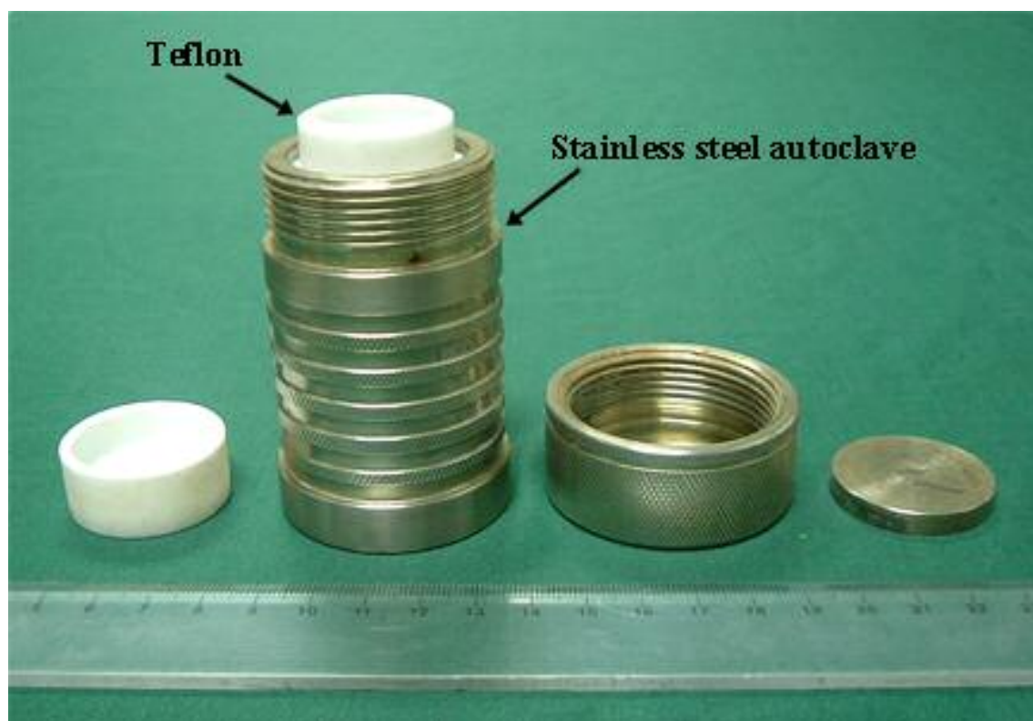
Figure S2. The photograph of the experimental setup, including a teflon vessel and a stainless steel autoclave.
