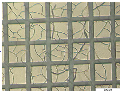
Figure S5. Optical images of gravure-printed CPB films with vapor-deposited Au electrodes; Optimized – PVP-EGOAc (100:50), Unoptimized – PVP-C 6 Cl (100:50). The scale bars indicate 200 \mu\text{m} .
