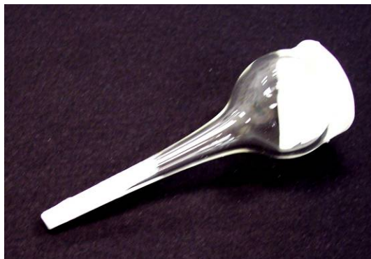
Figure 2. At the end of reaction the PTFE tape was undamaged and the tube could be reused.
