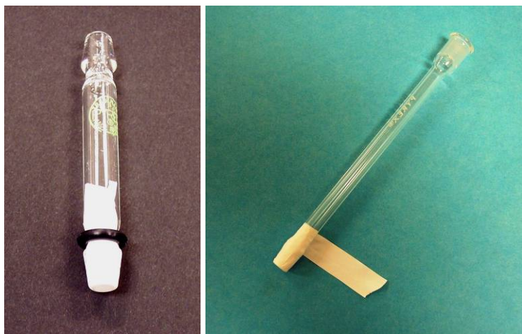
Figure 3. In some cases the PTFE tape had to be secured with a) an O-ring, or b) an additional PTFE wrap.
