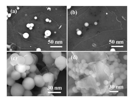
It was found that the attachment of  $TiO_2$  nanoparticles on GS is not significant in sample 1 (Fig. S4a, b) with only 5 hours oxidation, but the attachment of  $TiO_2$  nanoparticles is considerable in samples 2 and 3 with oxidation times higher than 10 hours (Fig. S4c, d). Combining this with the above XPS results, we deduce that the good attachment of  $TiO_2$  nanoparticles in samples 2 and 3 is due to the increase of residual oxygen-containing groups with long oxidation process.
