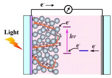
ITO TiO<sub>2</sub>/GS Dye Electrolyte Pt
