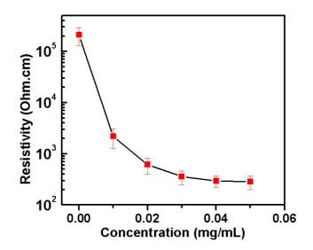
The resistivity of GS/TiO<sub>2</sub> films decreases continuously with increasing GS concentration and approaches  $2.85 \pm 0.87 \times 10^2 \ \Omega$ ·cm at GS concentration of 0.05 mg/mL.
