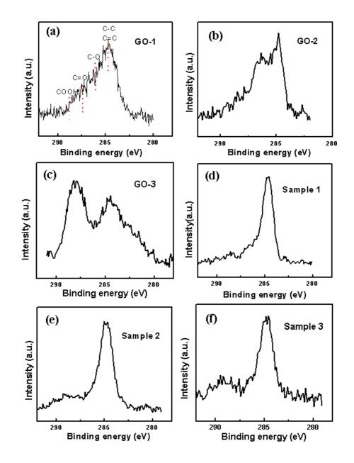
**3.** Figure S3 (a-c) The C 1s peaks in the XPS spectra of GO precursors from samples 1-3. (d-f) C 1s peaks in the XPS spectra of reduced GS from samples 1-3.
