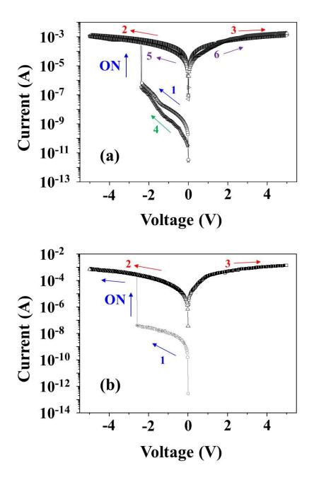
**Figure S1.** I-V curves of the ITO/ PPOXBPA(30 nm thick)/Al devices: (a) as-cast film; (b) thermally annealed film. The voltage was swept from 0 to -5.0 V.
