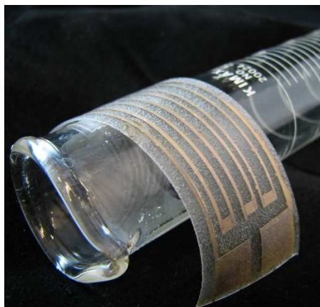
Figure S3. Optical image of silver electrode patterned produced by airbrush spraying the reactive silver ink onto an ethylene vinyl acetate substrate.
