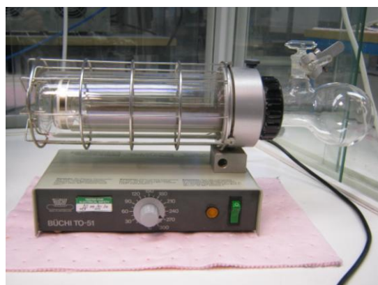
Figure 1. Commercially available Buchi TO-51 used for calcinating zirconium hydroxide.
