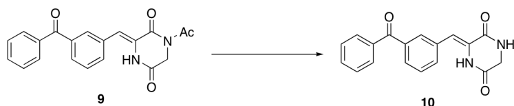
Scheme S2. Reagents and conditions: aqueous 28% \text{NH}_4\text{OH} , DMF, rt, 1 h.
