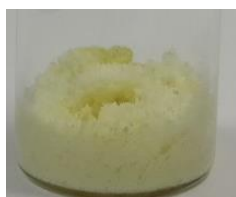
Figure S7. Photo of GPPCN/H 2 SO 4 paste (600 mg/mL), the intermediate state during the dissolution of GPPCN in H 2 SO 4 .
