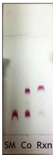
Figure S3. Normal phase silica TLC (5:5:1, EtOAc:CH 3 CN:H 2 O) comparison of crude 1 starting material (SM), the reaction mixture of 1 and 3 after 8 hours (Rxn), and the co-spot of both (Co).
