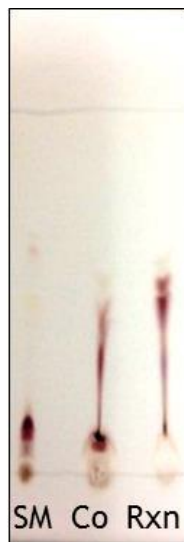
Figure S2. Normal phase silica TLC (5:5:1, EtOAc:CH 3 CN:H 2 O) comparison of crude 1 starting material (SM), the reaction mixture of 1 and 2 after 6 hours (Rxn), and the co-spot of both (Co).
