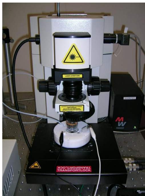
Figure S3. Schematic diagram and photograph of the electrochemical Raman spectroscopy system. The laser is not shown in the photograph.
