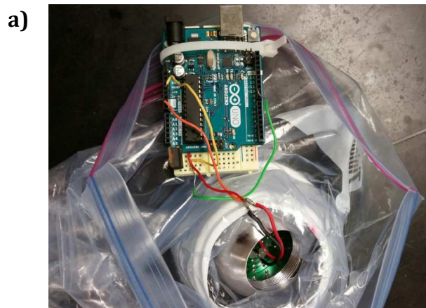
Figure S13. a) Internal Arduino setup, and; b) and incubator Arduino setup. For irradiations exceeding 12 hours, light sources were hard wired to a 12V AC power source.
