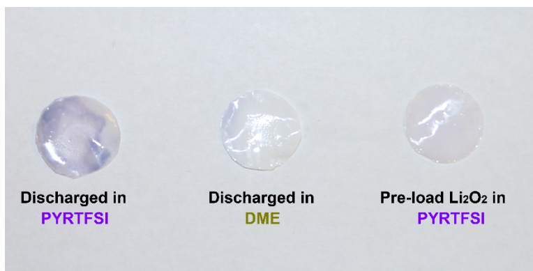
Figure S3: Detection of superoxide radical by nitrotetrazolium blue chloride. (A). Discharged in \text{PYR}_{14}\text{TFSI} ; (B) Discharged in DME; (C) Pre-load commercial \text{Li}_2\text{O}_2 in \text{PYR}_{14}\text{TFSI} .
