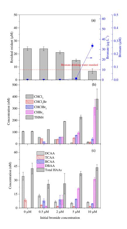
Figure S6. Effect of initial bromide concentration on formed bromate as well as bromine and chlorine in THMs and HAAs. Experimental conditions:  $[HOCl]_0 = 40~\mu\text{M}$ ,  $[Br^{-}]_0 = 0\text{-}10~\mu\text{M}$ ,  $[DOM] = 2.5~mg~L^{-1}$ ,  $[CuO] = 0.025~g~L^{-1}$ , pH= 8.6,  $T=21\pm1~^{\circ}\text{C}$ , reaction time = 8 h.
