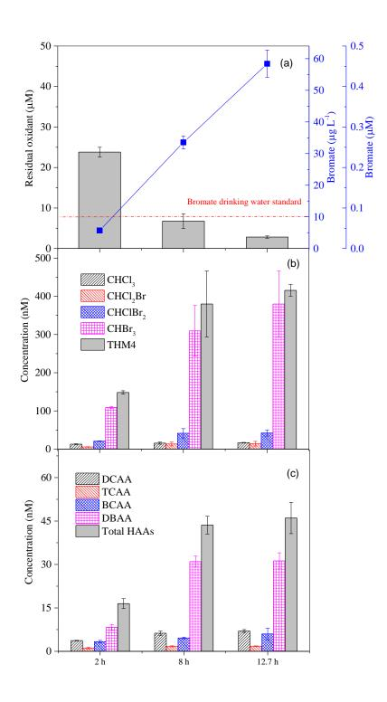
Figure S4. Effect of initial chlorine concentration on formed bromate as well as bromine and chlorine in THMs and HAAs. Experimental conditions: [HOCl] $_0=14\text{-}70~\mu\text{M}$ , [Br $^-$ ] $_0=10~\mu\text{M}$ , [DOM] = 2.5 mg L $^{-1}$ , [CuO] = 0.025 g L $^{-1}$ , pH= 8.6, T =21±1 °C, reaction time = 8 h.
