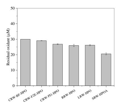
Figure S12. Effect of DOM type on oxidant decay and bromate formation in the presence of CuO. Experimental conditions: [HOCl] $_0$  = 40  $\mu$ M, [Br $^-$ ] $_0$  = 10  $\mu$ M, [DOC] = 1.3 mg C L $^{-1}$ , [CuO] = 0.1 g L $^{-1}$ , pH= 8.6, T =21±1 °C, reaction time = 2 h.
