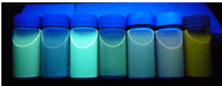
Figure S1. As-prepared reaction mixtures under irradiation with UV light. From left to right, these samples were produced by hydrothermally treating mixtures of p-phenylenediamine (0.2 g) with ethylenediamine (700 \mu L), 4,7,10-trioxa-1,13-tridecanediamine (700 \mu L), polyethyleneimine (700 \mu L), glucose (0.2 g), citric acid (0.2 g), L-threonine (0.2 g) and phosphoric acid (700 \mu L), respectively.
