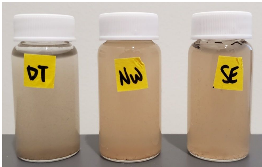
Figure S36. Picture of actual, unfiltered samples from the Houston Hurricane Harvey flood waters (from left to right: downtown Houston, 5 miles northwest of Houston, and 5 miles southeast of Houston) analyzed with the reported device
