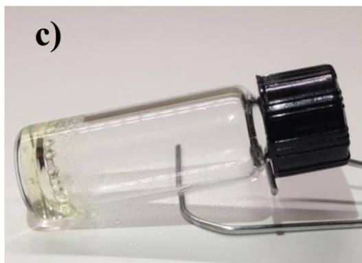
Figure S8. Control experiments for the formation of a dynamic hydrogel via transthioesterification reactions a) in neutral aqueous media, b) in acetate buffer at pH = 4, c) hydrogel after the treatment with excess thiol (linear PEG-thiol 800, 10 equiv.) dissolved in acetate buffer (25 \mu L) at pH = 4 for 12 hr. d) degradation of hydrogel after the treatment with excess thiol (linear PEG-thiol 800, 10 equiv.) dissolved in neutral aqueous media (25 \mu L) for 12 hr. Reaction conditions: monomer 3a (1.0 equiv, 0.5 \mu mol), PEG-thiol 10'000 (2.0 equiv, 1.0 \mu mol), in 75 \mu L of aqueous media (20 wt% solid content), at ambient ( \sim 25°C) for 12 hr.
